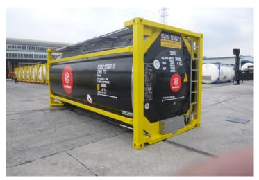
of the tank, high-capacity digital thermometer, a thermowell to measure the product temperature in the middle of the tank, top valve and siphon tube and collapsible handrails.
